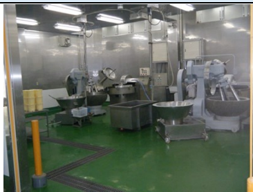
Blender room with two 250 kg cutters
